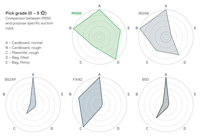
Testing performed using low vacuum flow with COAX® MICRO Si cartridges.
