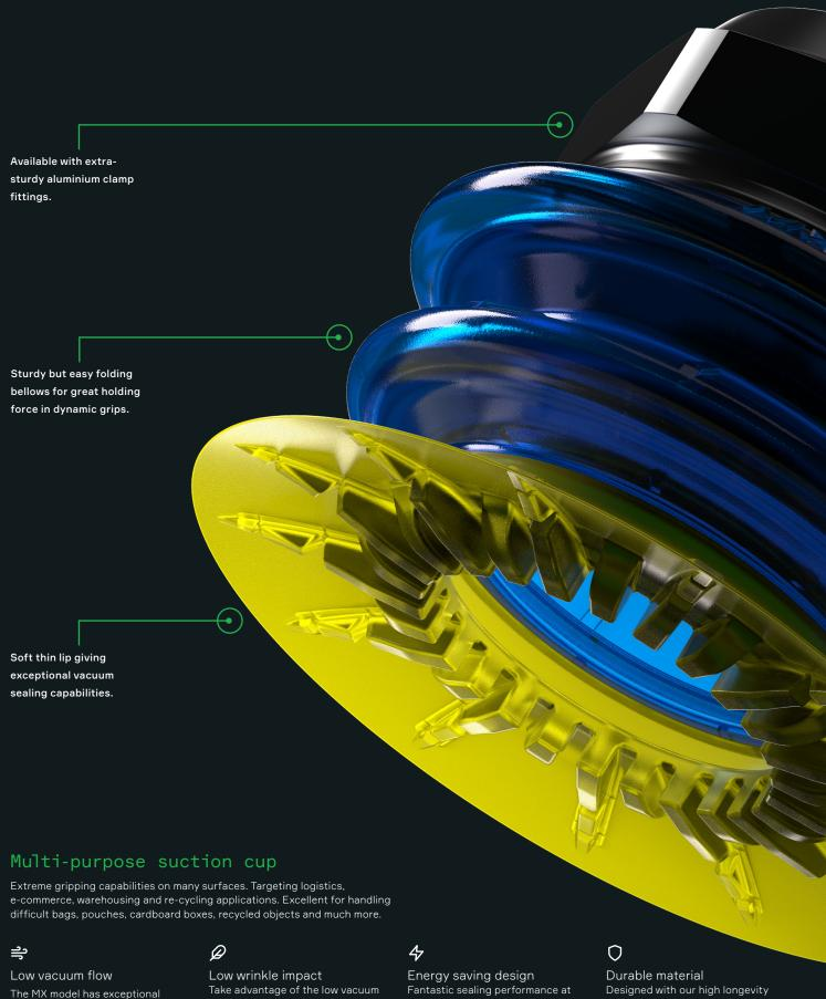
The MX model has exceptional sealing capabilities at lower vacuum levels. There is less vacuum flow needed, even on difficult objects. This makes it a perfect fit for small vacuum systems such as piCOBOT®.
